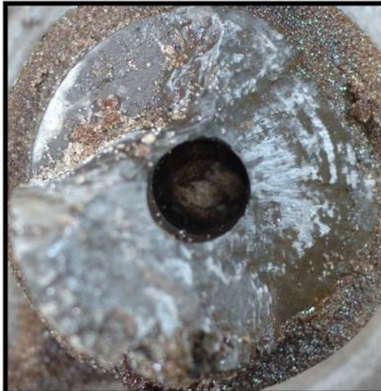
Photo 2 - Shallow Pleistocene shale drilled with 0.5 Aw oil mud
