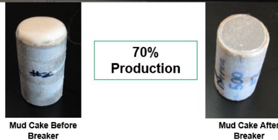
Figure 2: Formation Response Tester; Mud Cake on Core Face Before and After Breaker Soak Resulting in 70% Production
