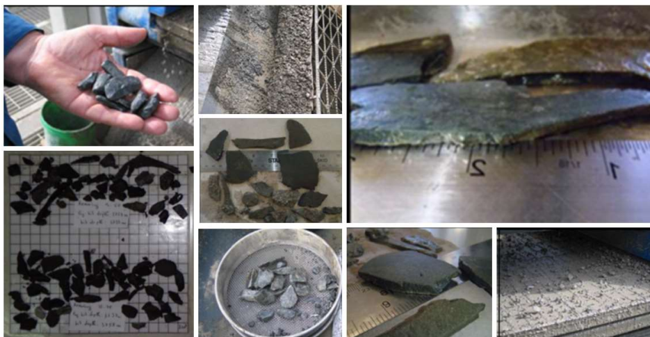
Figure 2: Recovered cavings (angular, splintery & blocky)
