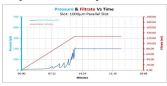
The results showed that the Background LCM blend used had the ability to seal the 1,000micron slot up to a max differential pressure of 200 psi in <14 minutes. The amount of fluid that passed upon reaching maximum differential pressure was <130 ml. Once maximum pressure was achieved it was held for ~10 minutes for observation. The seal did not break back during the entire test.
